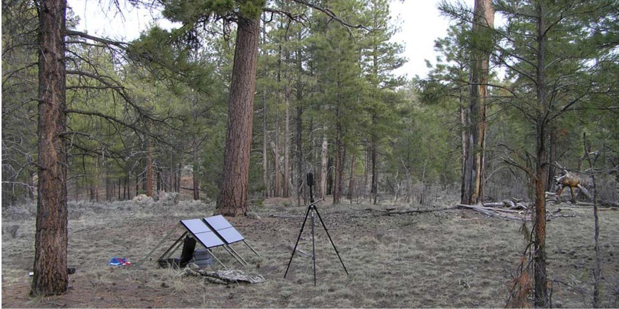
**Figure 2. Sound data collection equipment. The laptop, sound level meter, and gel cell batteries are underneath the solar panels.**
