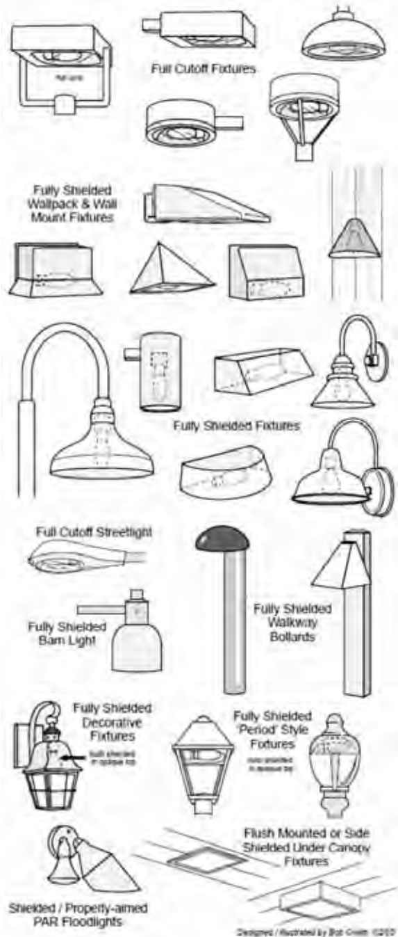
Figure 65. Examples of fully shielded luminaires. (IDA-MLO 2011)
