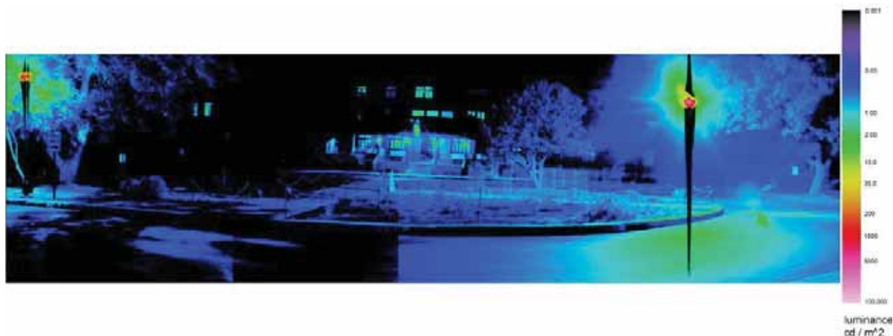
Figure 38. Panoramic luminance map of the front entrance and drive-up area of El Tovar Hotel.
