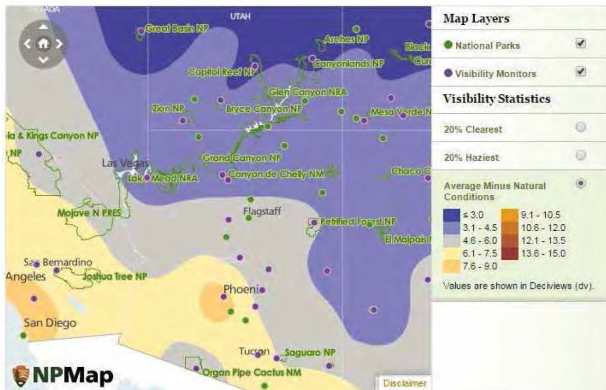
Figure 5. A regional visibility map showing the average minus the natural conditions in deciviews (dv). Areas of higher visibility are indicated in blue, areas with higher anthropogenic haze are indicated in tan, browns, and reds. Data viewer available at: http://www.nature.nps.gov/air/maps/AirAtlas/visibility.cfm
