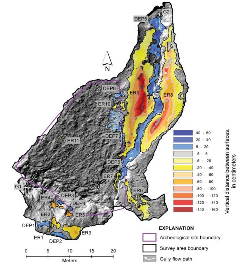
*Lidar map showing topographic change that occurred between 2007 and 2010 at one study site, showing erosion (warm colors) and deposition (cool colors). Image and data from Brian Collins, USGS.*
