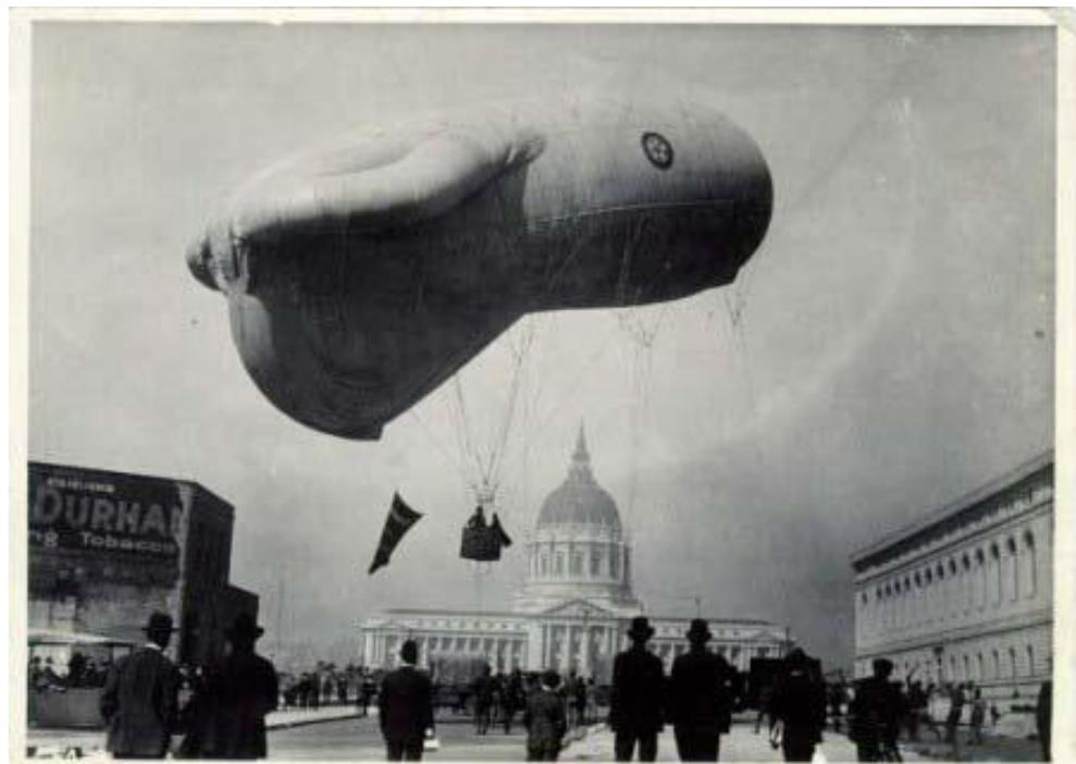
shape) consisted of a hydrogen-filled body equipped with fins that provided stability in rough air, and a suspended wicker basket that held a two-man crew. Communication between the observers and the ground crew was via a telephone cable spliced onto the mooring line. Before long, the Americans began manufacturing their own version of the French balloons, which the army designated the Type C-3. During 1918-1919, nearly a thousand C-3s were manufactured in the U.S.<sup>3</sup>
