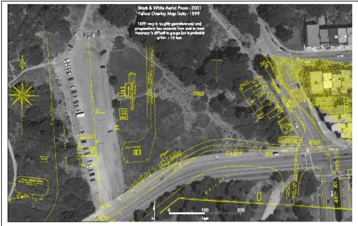
**Figure 60.** Overlay showing 1899 structures in the Triangle and 2001 existing conditions. The original Ferries & Cliff House depot and Ocean Terrace development are at right, and the Scenic Railway and Firth Wheel are at center. Also note the cluster of small concession stands lining “Cliff Avenue” east of Merrie Way. (Golden Gate National Parks Conservancy)
