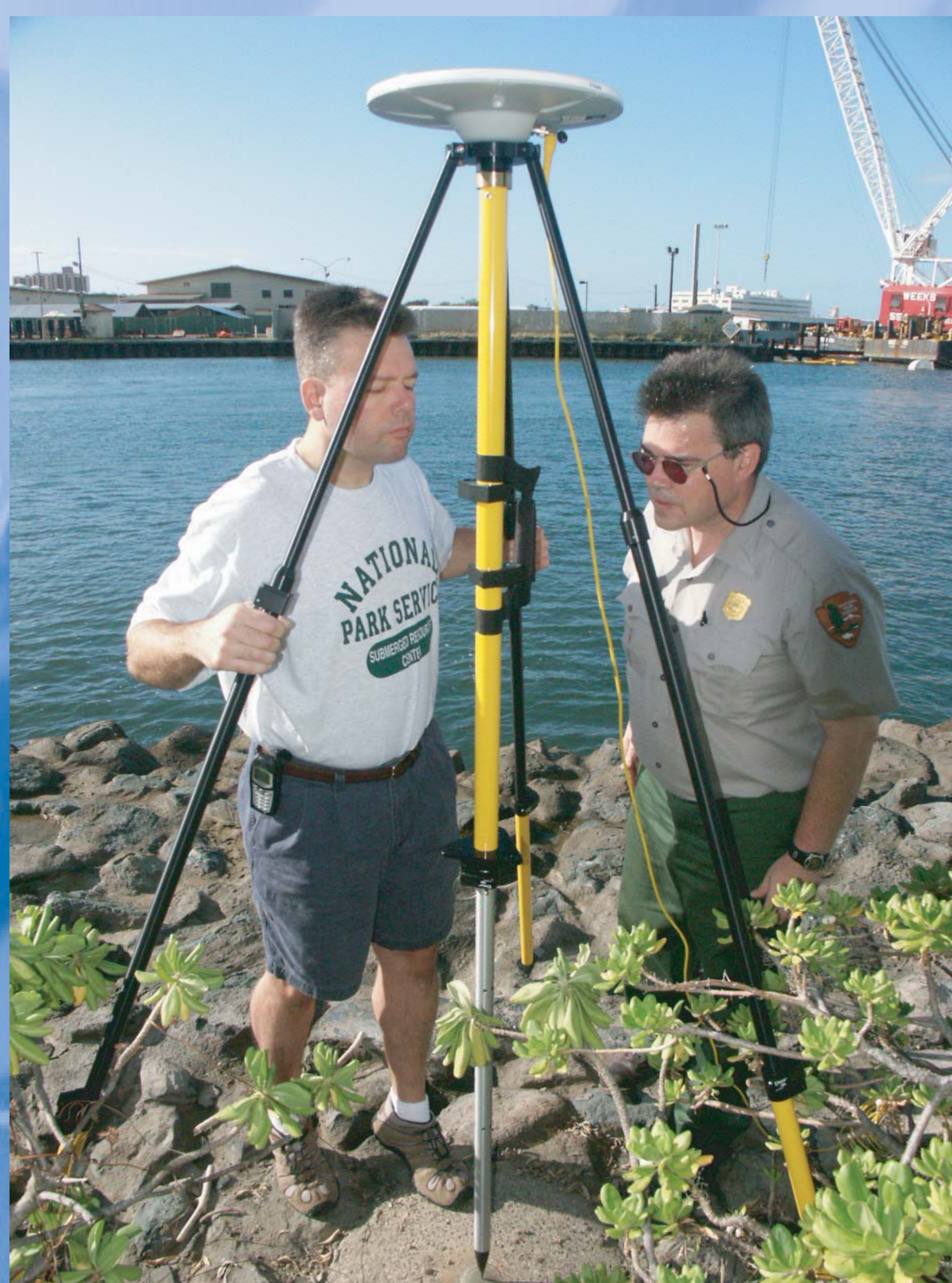
Trimble's Brian McInnis and NPS surveyor Mark Duffy setting up 5700 base station receiver near park headquarters in 2003. (NPS Photo by Tim Smith)
