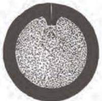
**Shell** also used a timed fuse with the intent of having the ammunition explode over the heads of the enemy soldiers, sending small, sharp pieces of the shell in all directions. (Actual diameter equalled approx. 3.5 inches)
