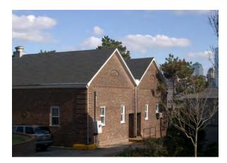
**Building 109** is an open floor plan building constructed in 1945. It is situated in a prime location adjacent to Soissons Landing. The double gable building is brick on masonry bearing walls. The roof is in poor condition and the structure is a shell only with some structural concerns. Floors: 1
