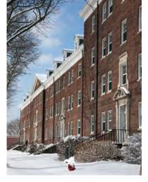
**Building 12** is a 140,000 square foot building broken into fifteen sections, each containing six three-bedroom apartments. This building includes attic and basement. The structure is brick on reinforced concrete with a slate roof. The building was constructed in 1931 from the designs of architects McKim, Meade and White. Floors: 3 plus attic and basement Square feet: 140,000
