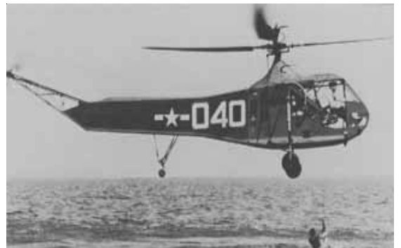
The first helicopter rescue winch is demonstrated by Coast Guardsman Sergei Sikorsky, the son of its inventor Igor Sikorsky, on land (left,) and in Jamaica Bay off Floyd Bennett Field in 1944. This device proved invaluable in the air - sea rescue role.
