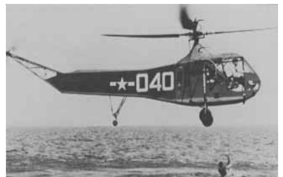
The first helicopter rescue winch is demonstrated by Coast Guardsman Sergei Sikorsky, the son of its inventor Igor Sikorsky, on land (left,) and in Jamaica Bay off Floyd Bennett Field in 1944. This device proved invaluable in the air - sea rescue role.
