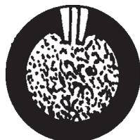
Shells are hollow, with a charge of gunpowder inside. The powder is ignited by a timed fuse, which lights when the gun is fired. Shells are generally used to set fires.
