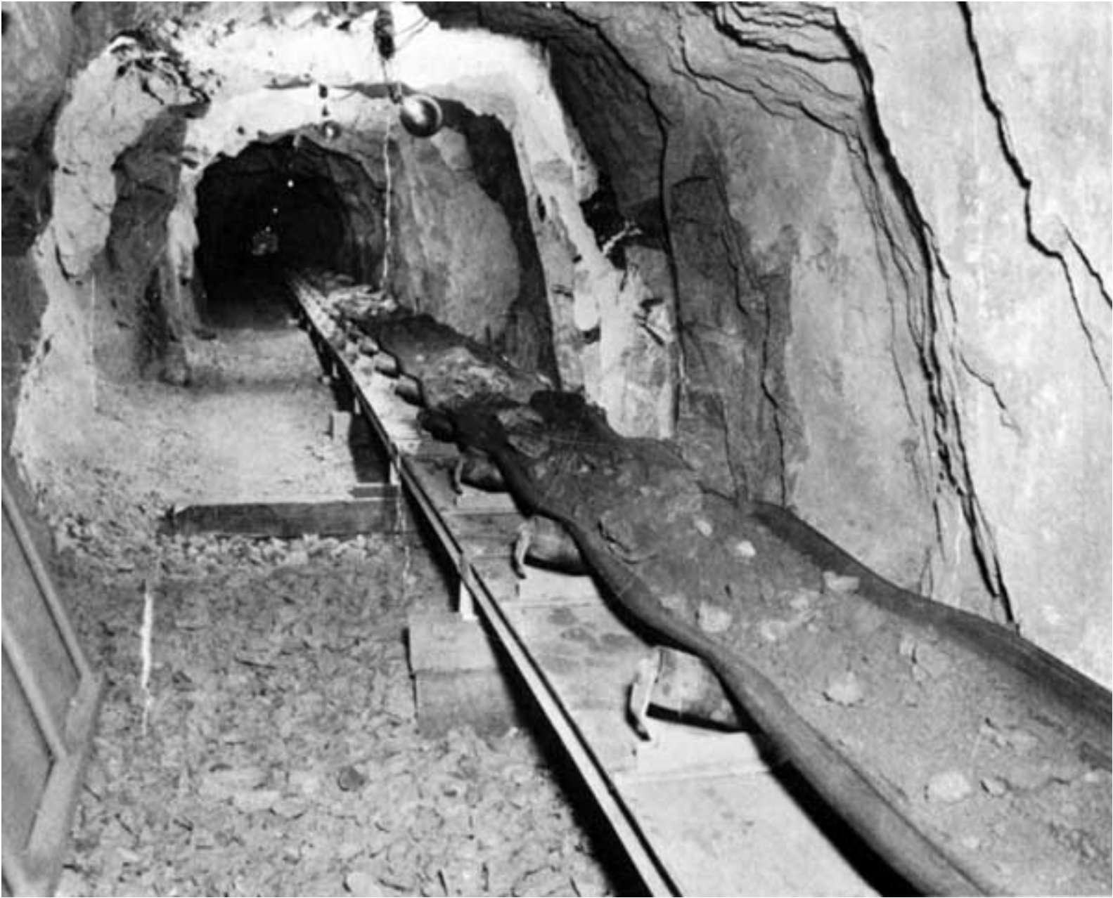
Figure 8. Fluospar Mine Number 21, showing conveyor belt system. Fluorspar was a multi-purpose mineral used in the manufacturing and hardening of steel, paints and acids. Photograph taken about 1948, from the collection of Mrs. Dovey Bright.
