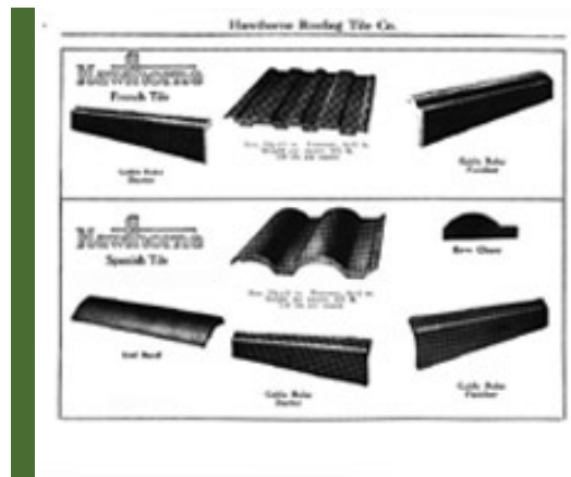
Chicago-based Hawthorne Roofing Tile Company originally manufactured its tile from slabs by a hand-process. These concrete roofing tiles depicted in the 1929 Sweet's Architectural Catalog imitated French and Spanish clay tiles. They were produced with automated power-driven equipment, and the colors were impregnated on the tile surface. ( Sweet's Architectural Catalogue, 1939 . Courtesy of the Sweet's Group, McGraw Hill Companies, Inc.) [click image for larger view]
