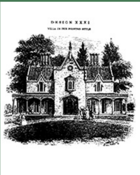
Downing describes the chevron patterned roof of his Design XXXI, "Villa in the Pointed Style," from The Architecture of Country Houses published in 1850: "The roof may be covered with zinc laid on a ribbed sheathing, without soldering so as to allow it to expand and contract without detriment." (Courtesy of The Athenaeum of Philadelphia) [click image for larger view]
