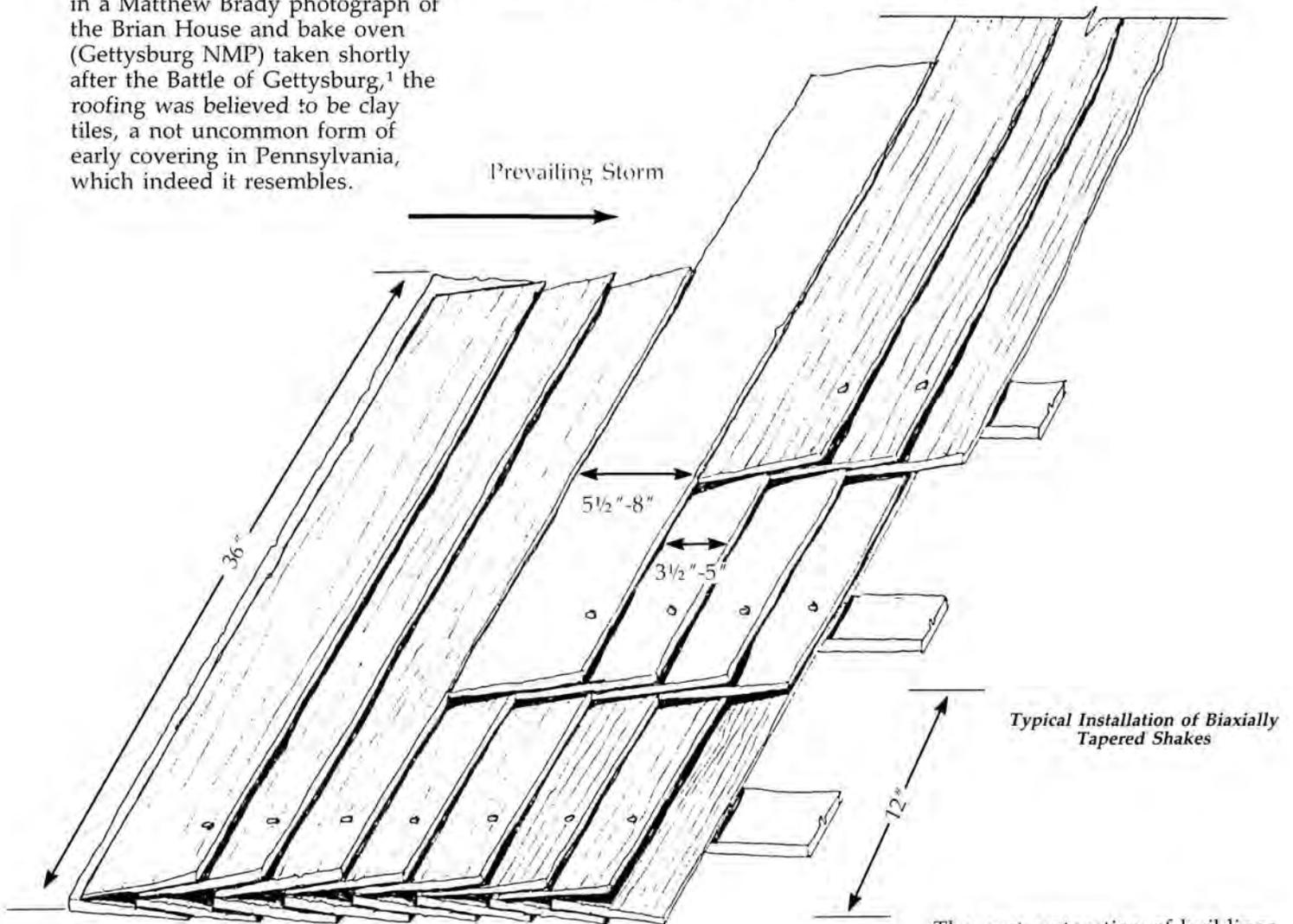
Reexamination of the photograph led, however, to the eventual recognition that the roofing was not tile, but in fact drawn shakes laid in what was at first considered a highly unusual manner. Subsequent archival and field research has revealed that this roofing type, herein called biaxially tapered shakes for lack of a better name, was common in areas of Germanic settlement through the latter part of the 19th century.
