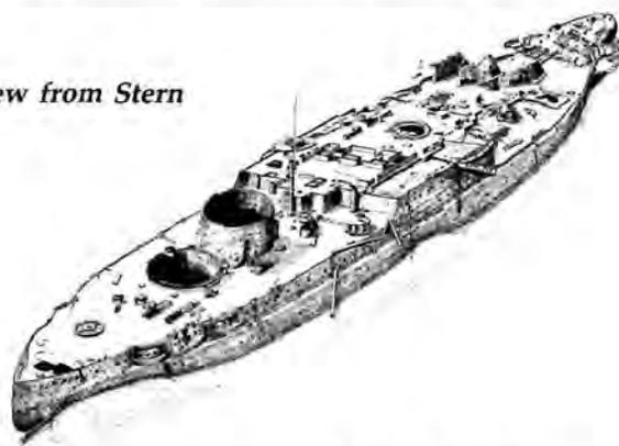
Drive shafts, propellers, rudder and hull at the turn of the bilge is projected by dotted lines. *Arizona's* stern configuration was that of a cruiser with one large rudder. Lower hull spaces were boiler-feed water tanks, potable water supplies, and fuel oil bunkers. Toward
