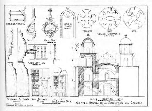
A typical sheet of (28) drawings by the NPS architects, following measurements made during the 1935 expedition. In addition to the large structural forms, they also recorded decorative details for possible use at the Tumacacori National Monument Museum. (Hollis Phototechnics, photo, courtesy of N. J. Bleser)
