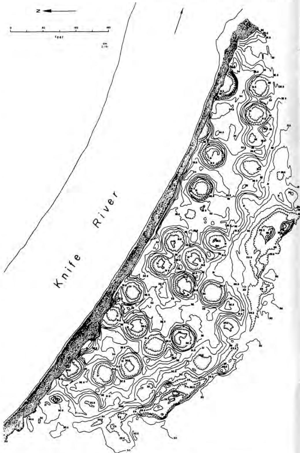
Contour map of the Sakakawea Village, produced photogrammetrically from aerial photographs. The contour interval is six inches.
