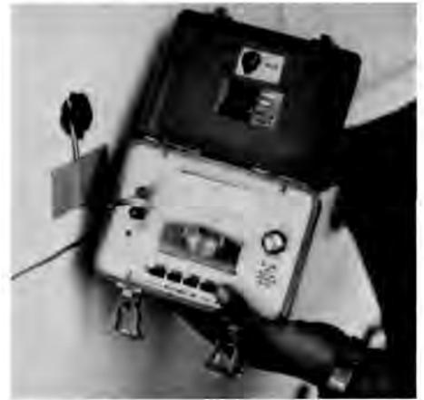
Photo 6. Moisture cells were installed around the perimeter of the René Beaugard House and on one of the columns. These cells, 22 of them, have been periodically read with a moisture meter to chart the success of the treatment. Photo by Williamsport Preservation Training Center, NPS.
