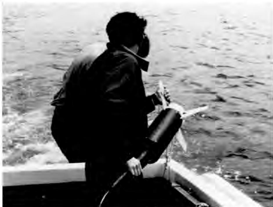
Deployment of magnometer sensor head from stern of survey vessel, Drakes Bay, Point Reyes National Seashore, CA.
