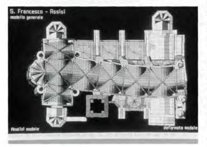
forces. This results in local amplifications and acceleration in case of north-south seismic forces larger than that in the center of the city of Assisi. These considerations bring us to take into account a possible maximum ground acceleration of around 0.3 to 0.35 g, in the perpendicular direction with respect to the basilica nave (longitudinal axis).
