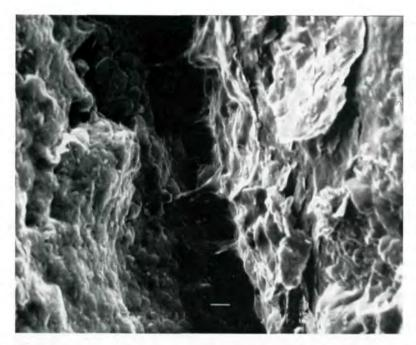
Rhoplex<sup>®</sup> strands in soil-mortar sample at 5,000X. Photo by Bob Hartzler. coating, ruptured as the clays in the soil expanded and contracted.
