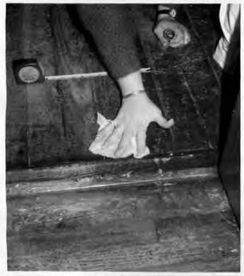
A dust wipe test can identify the active presence of lead. A moist towelette is used to collect dust and then is analyzed in the laboratory. If a property is freshly painted and well maintained and floors have been thoroughly washed and wet vacuumed, a dust wipe test can verify that it is lead-safe.
