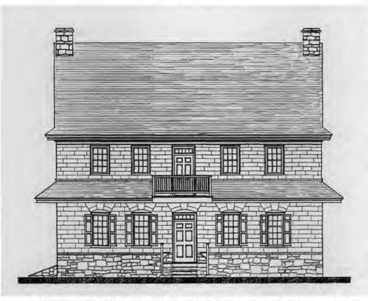
Fig. 1. Muhlenberg House, Principal Facade, c. 1755. The Muhlenberg House is 31'-0" x 39'-0" in plan. The red sandstone is laid in a coursed ashlar pattern on the front facade above the water table. All other facades are laid in a rubble pattern. Drawing by Christina Henry, John Milner Architects, Inc.
