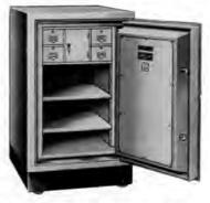
Fig. 5. Single door fire resistive safe for paper records. Unit shown is rated Class 350, 2-Hour. Source: Meilink.
