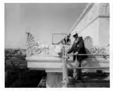
HABS architect Mark Schara (left) and HAER photographer Jet Lowe are captured in an image taken by the photogrammetric camera mounted at the end of a photo boom at the top of the Lincoln Memorial scaffolding. The empty frame provides four coordinates of known separation, used to provide scale and orientation during the digitizing process. The resulting drawing is shown at right.
