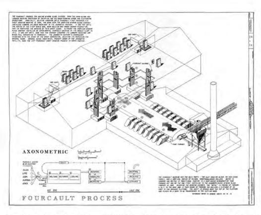
Fourcault process for making window glass, patented by Belgian inventor Emile Fourcault in 1904. Installed at Jeannette in 1928. Delineated by Cecilie Trolle and Sanford Garner, 1992.
