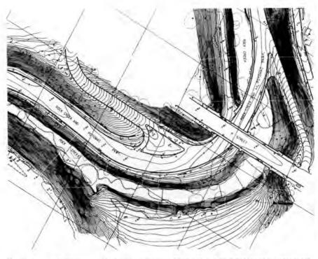
Detail of area as digitally mapped, showing 1' contours, tree bases, and probable canopies. Air Survey Corporation, 1992.
