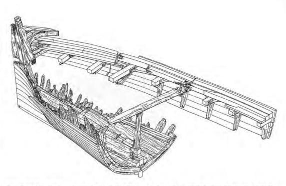
Axonometric drawing of *Snow Squall's* hull shows the distinctive bow profile of a clipper ship. Delineated by Karl Bodensiek, 1992, HAER.
