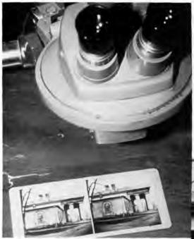
1. Historic photos, such as this circa 1869 stereopair photograph, were used to document the configuration of the **Arlington House** roof during Robert E. Lee's time. A spe cial microscope (left) affixed with a 35mm camera was used to produce magnified sections of the photographs (right) to provide the details for restoration.
