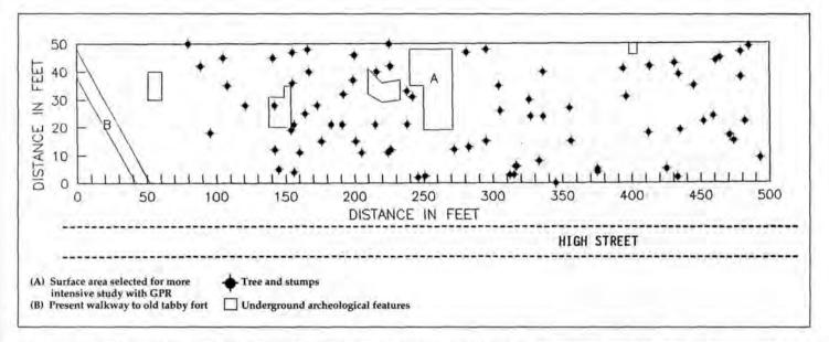
Figure 3: Diagram of 500'x 50' rectangular grid established over study plat area, southwest of High Street, on Old Dorchester State Park. Area "A", near the center, was selected for a more intensive survey with GPR.
