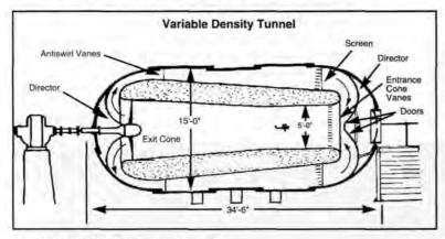
Drawing of Variable Density Wind Tunnel
