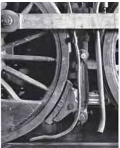
ABOVE: LOCOMOTIVE WHEEL AND BRAKE SHOE. RIGHT: WORKERS AT THE EAST ELY SITE TAKE ON THE HEAVY WORK OF THE STEAM ERA.
