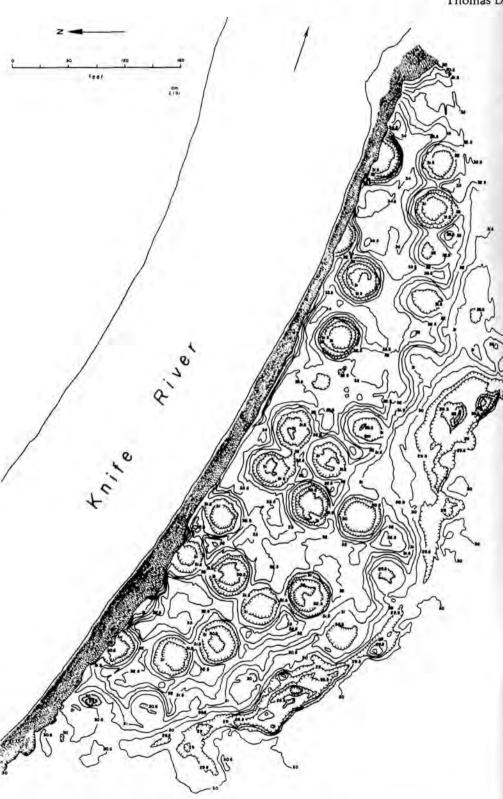
Contour map of the Sakakawea Village, produced photogrammetrically from aerial photographs. The contour interval is six inches.
