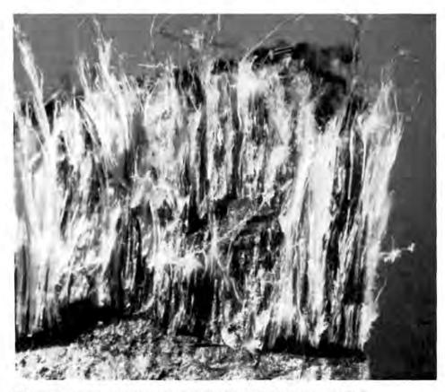
This macrophotograph of chrysotile asbestos (magnified 8 times) illustrates the dual nature of the mineral. Mined as a solid material (lower portion of photograph), this type of asbestos can be separated into fibers (upper portion of photograph) through processing. Because these fibers can easily be suspended in the atmosphere and are hazardous when breathed, most building products containing asbestos have been banned in the United States. Photo courtesy of the Bureau of Mines.
