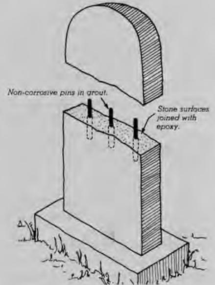
**Adhesive:** There are two types of epoxy resin used in this type of repair. Both are unaffected by moisture. The adhesive used to hold the pins is a high-strength (high modulus) epoxy used for structural repairs and the setting of bolts. It is fairly rigid. Masonry grout can also be used to set the pins, as seen in the tombstone example. A more flexible adhesive epoxy, a low modulus compound, is used to bind the two fragments together.
