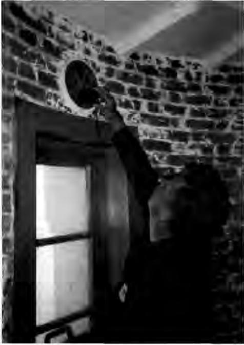
Art Corliss using a velocimeter to measure the draft through an air intake vent.
