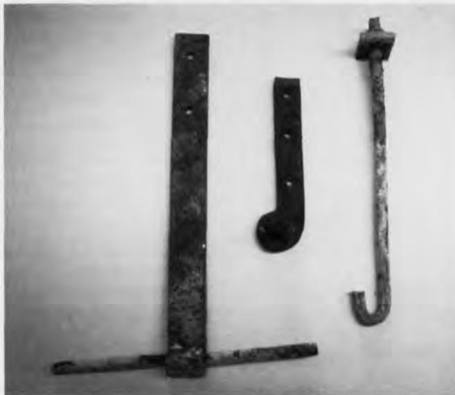
Fig. 2. Brick anchors made of iron, from left to right:
