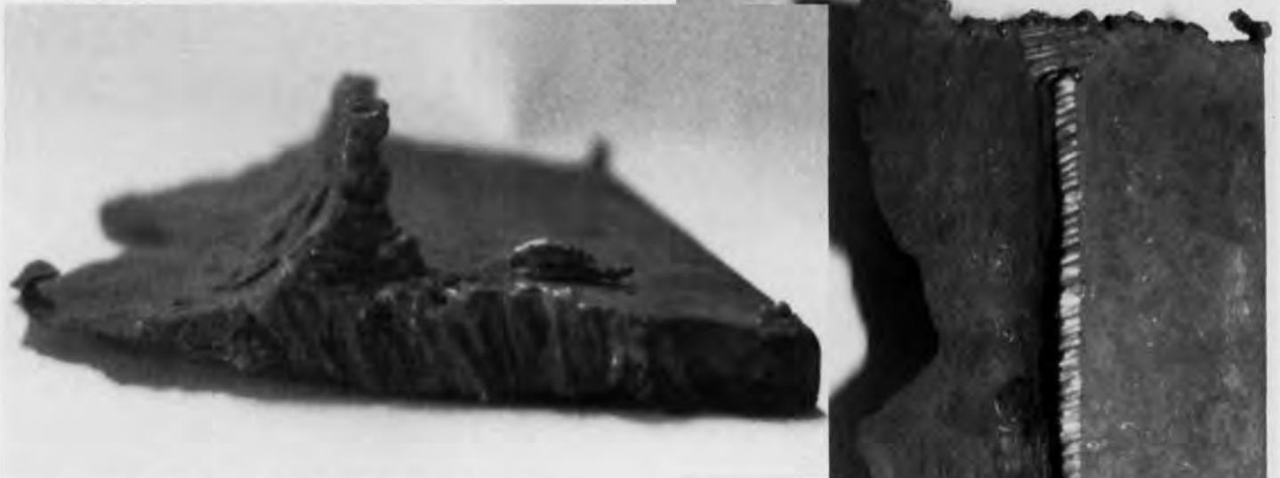
Fig. 1. Two views of a steel flange (c. 1891) from the structural framing at Carnegie Hall. Flange displays a fully corroded surface at one end and a non-corroded surface at the other. Photo by Marie Ennis, P.E., courtesy of Robert Silman Associates files.
