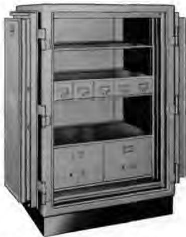
Fig. 6. Double door fire resistive safe for paper records. Unit shown is rated Class 350, 1-Hour. Source: Meilink.
