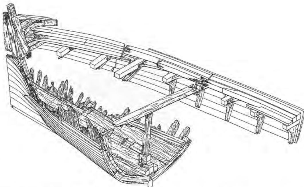
Axonometric drawing of *Snow Squall's* hull shows the distinctive bow profile of a clipper ship. Delineated by Karl Bodensiek, 1992, HAER.
