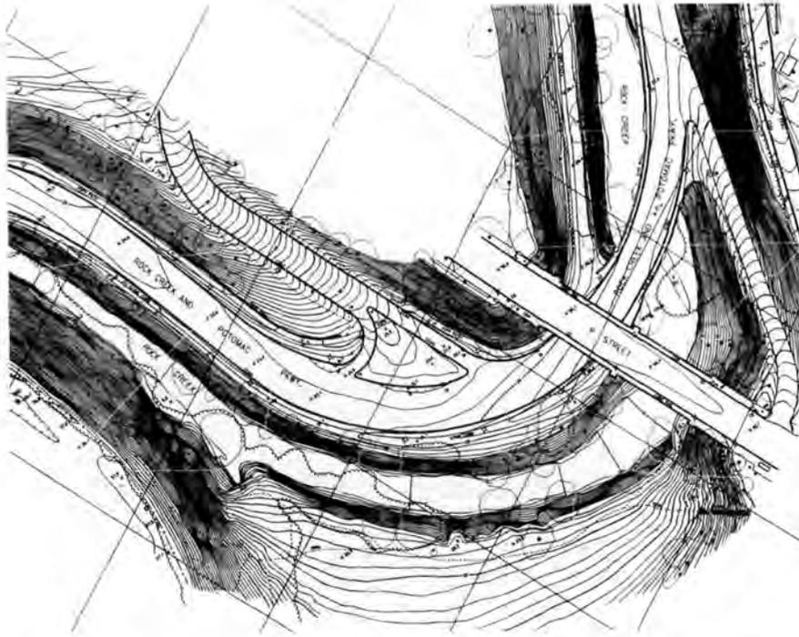
Detail of area as digitally mapped, showing 1' contours, tree bases, and probable canopies. Air Survey Corporation, 1992.
