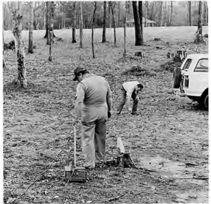
Figure 1: Photograph of ground-penetrating radar antenna being pulled by park superintendent, Charles Cumbee, along grid line at Old Dorchester State Park. Park ranger, Danny Dewees, is assisting with the antenna power cable to help Mr. Cumbee maintain a consistent speed with the antenna across the surface.
