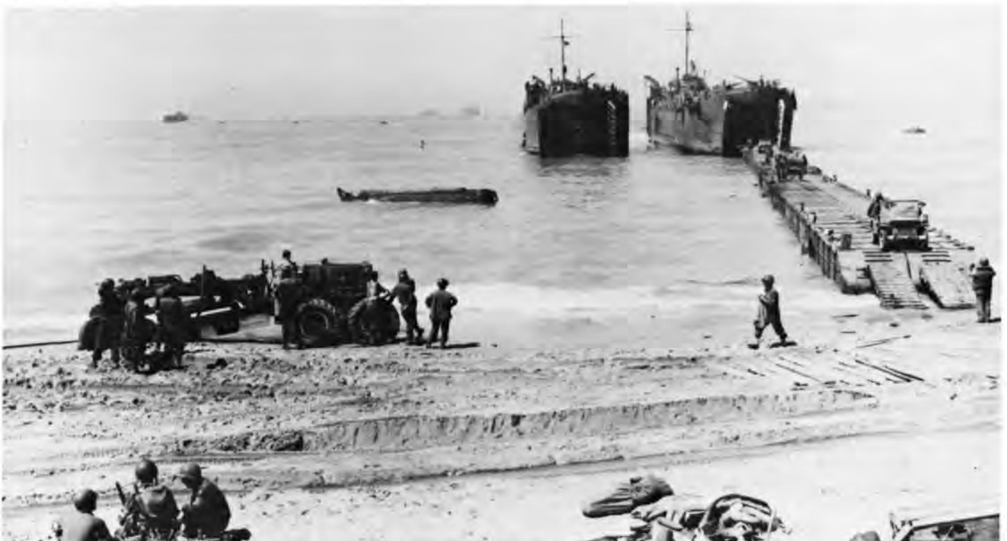
Landing Ships Tank (LSTs), with pontoon, unloading at Scogliatti Beach, Italy, July 10, 1943. LSTs, carrying vehicles, tanks and heavy materiel, brought along pontoon causeways, across which they could unload on the shallow beaches. This was the first use of LSTs and pontoons in combat. Bureau of Aeronautics photo courtesy of Robert L. Clifford.
