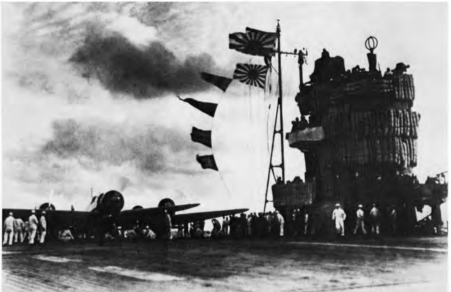
Readying for takeoff A6M2 (Model 21) Reisen fighter aircraft are prepared by flight deck crew for the second wave attack. This image was taken probably just before 7:00 a.m. aboard the Japanese carrier Akagi . Note battle flag array, rolled splinter matts, and dotted line stripes used by the pilots to guide takeoff and landing on a pitching deck.
