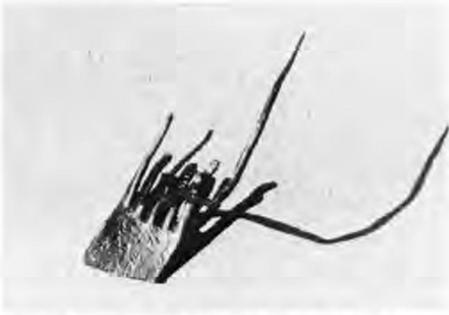
Fragment of a Nail Plate Which Had Been Partially Run Through a Slitting Mill at the Saugus Iron Works, Saugus, Massachusetts, ca. 1650.
