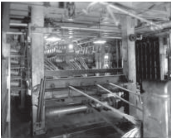
This photograph shows the bobbins with the yarn twisting into three strands and part of the forming machine.
