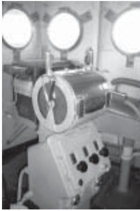
Engine room telegraph
