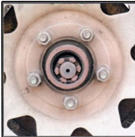
Right-Rear Spindle with Missing Dust Cap
