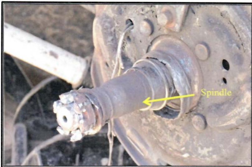
Damaged Right-Rear Spindle
