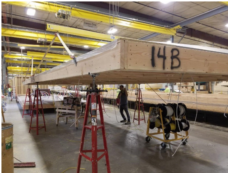
FIGURE 6 - WORKERS PREP PLUMBING AND ELECTRICAL IN FLOOR FRAMING AT FACTORY.
