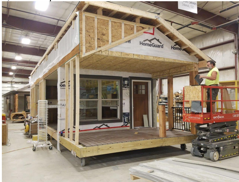
FIGURE 5 - TWO-BEDROOM MODULAR CONSTRUCTION IN FACTORY.
