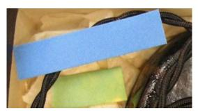
Figure 1.Blue A-D test reference strip above reacted green/yellow A-D strip
