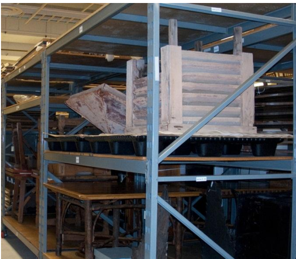
Figure 7.14. Racks for Large Objects. Slotted angle iron is used to construct racks for large objects.
