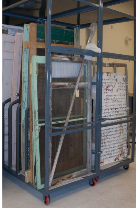
Figure 7.13. Rolling Unit for Large Objects. Movable custom designed storage equipment fabricated from slotted angle iron.
