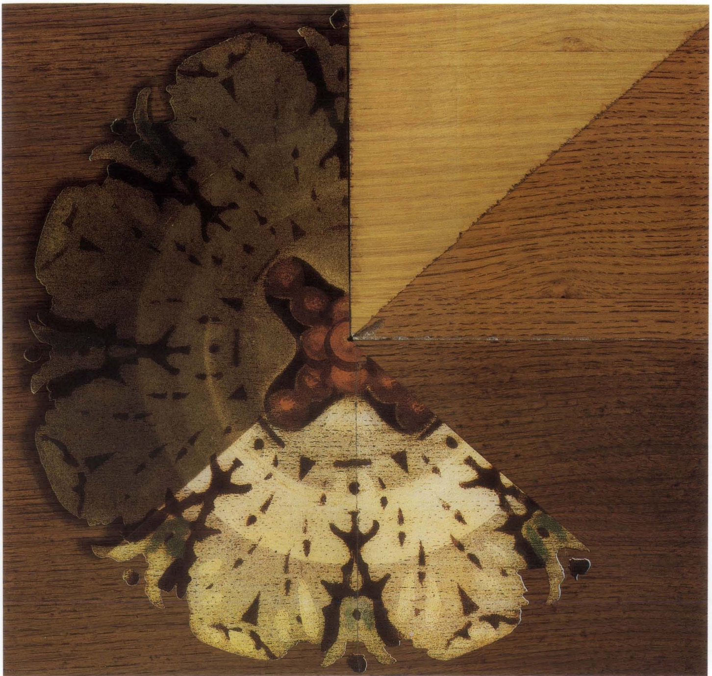
5. This demonstration model shows the various stages involved in finishing the ceiling panel. Starting with the raw wood panel in the upper right corner (1) and moving clockwise, a penetrating stain was applied (2) that matched the historic stain. A tinted varnish, or sealer, (3) was then applied to ready the backing panel to receive the decal (4). Two coats of acrylic sealer were used to protect this "cleaned" condition. The next 3 steps (5, 6, 7) produced the "aged" appearance with tinted varnish layers sprayed on using cardboard masks to produce the proper tones. A top coat of clear varnish (8) provided the final protective layer. Photo: Dell Corporation.
