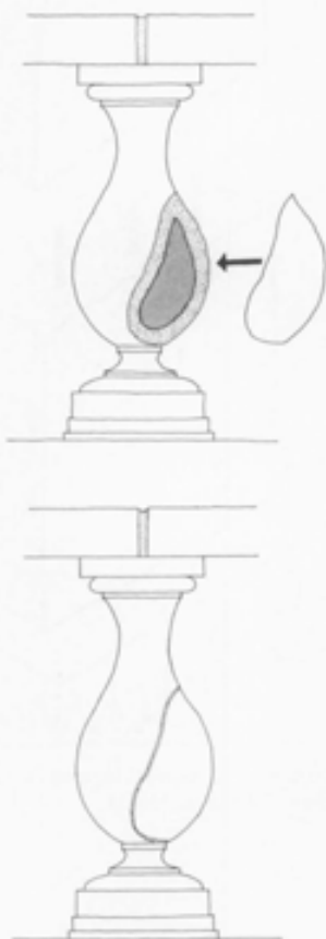
Epoxy repair of broken terra cotta baluster in which epoxy is applied to the break. The broken piece is reattached and the joint smoothed so repair is not visible. Illustration: Christina Henry.
