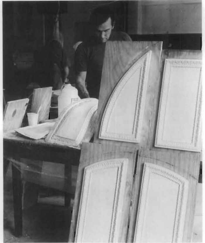
Figure 170. Plastic Patterns. Historically, most patterns for casting iron were carved from wood and pressed into sand to form molds. For the recasting of the iron shutters of the West Virginia Independence Hall, an attempt to use plastic patterns met with only limited success. How the original shutters, with their deeply undercut, beaded molding were cast in one piece is not known. To achieve the same effect in the restoration, the beaded molding of iron had to be cast separately and applied to the replicas. The patterns are mounted on plywood to give them enough rigidity so they may be hammered into the sand to form the molds. (West Virginia Independence Hall Foundation)
