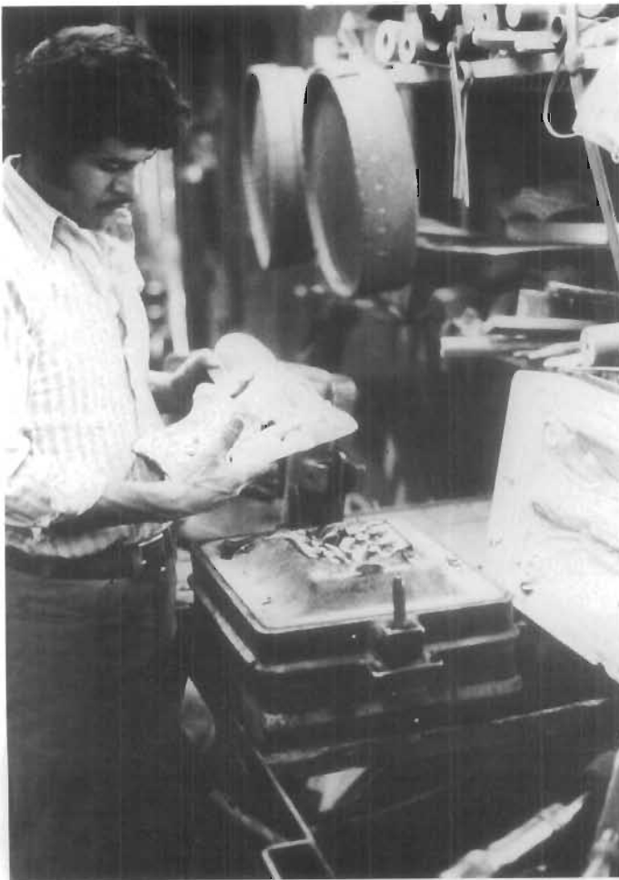
Figure 171. Sand Mold. The pattern has been pressed or hammered into the sand to form an impression or mold. Special casting flasks or boxes are used to hold the sand. Only one flask or box is required for an open mold which produces a casting with a flat top. To cast a piece with relief on both top and bottom requires two flasks stacked and bolted together. (Steven T. Baird)
