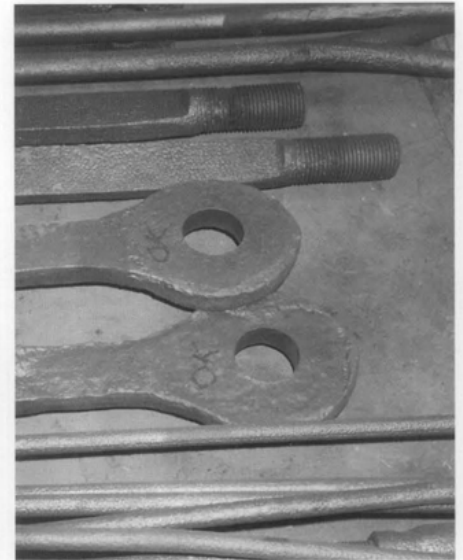
Figure 7. The pieces were disassembled in the shop, then cleaned of rust and paint. The worn condition of the eye bars can be seen in the center of the photograph. Photo: Beta Engineering.
