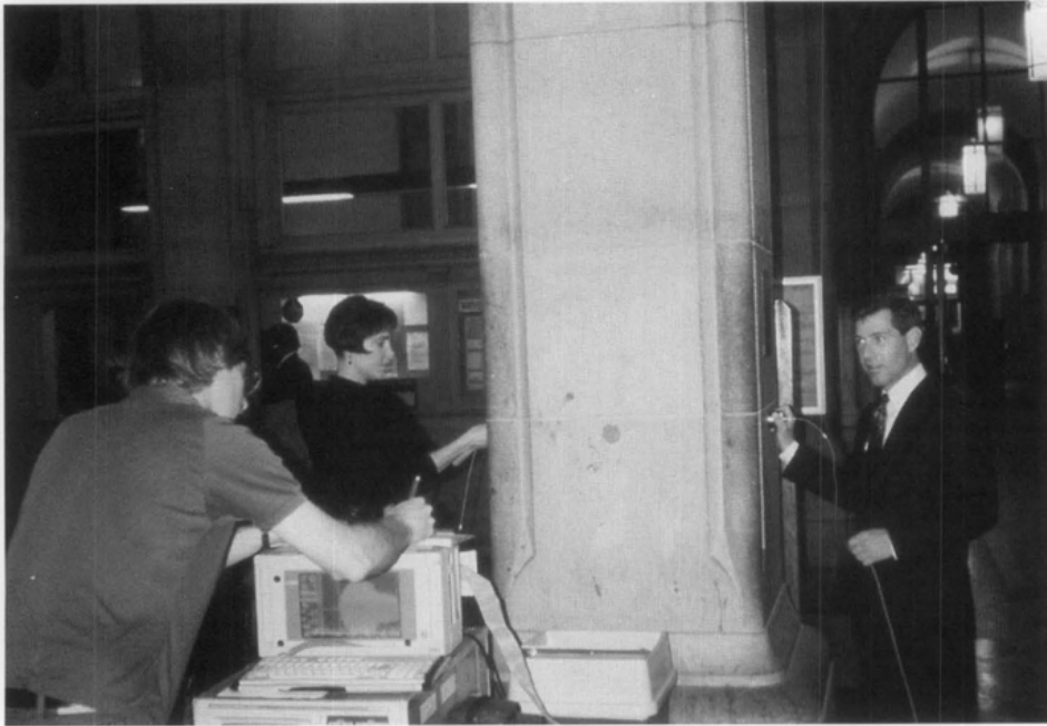
Fig. 5. Ultrasonic pulse velocity is being used to obtain characteristic wave velocities for granite. A transmitter is placed on one side of the column and a receiver on the opposite side. Photo: Andrea Lazarski.
