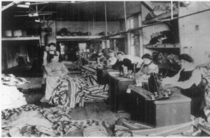
Figure 4. This 1892 photo shows the canvas sewing room of a large awning manufacturer. The wide variety of custom sizes and shapes, and the natural shrinkage of canvas demanded considerable skill in measuring, cutting and sewing. Photo: The Astrup Company.
