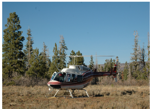
Type III helicopter used for aerial ignition
