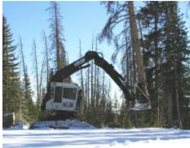
Contract feller/buncher removing hazard trees in winter.
