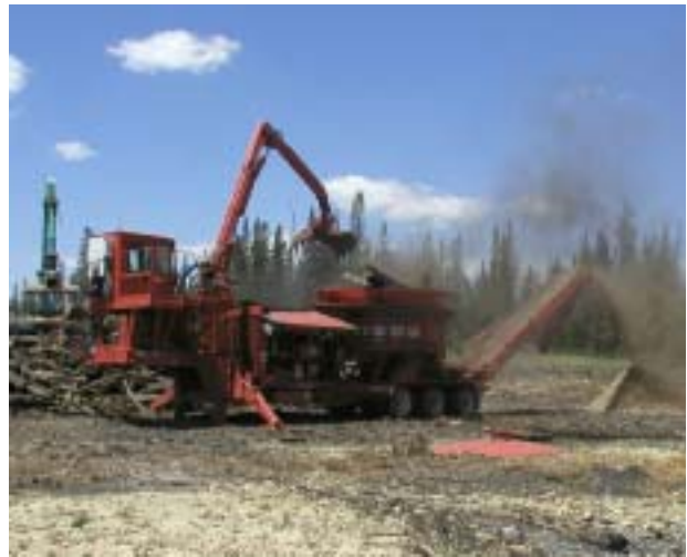
Contract tub grinder making wood chips from large slash.
